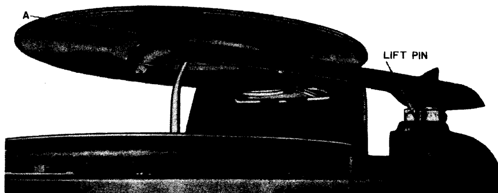
Fig. 11. Tone Arm Height Adjustment.
